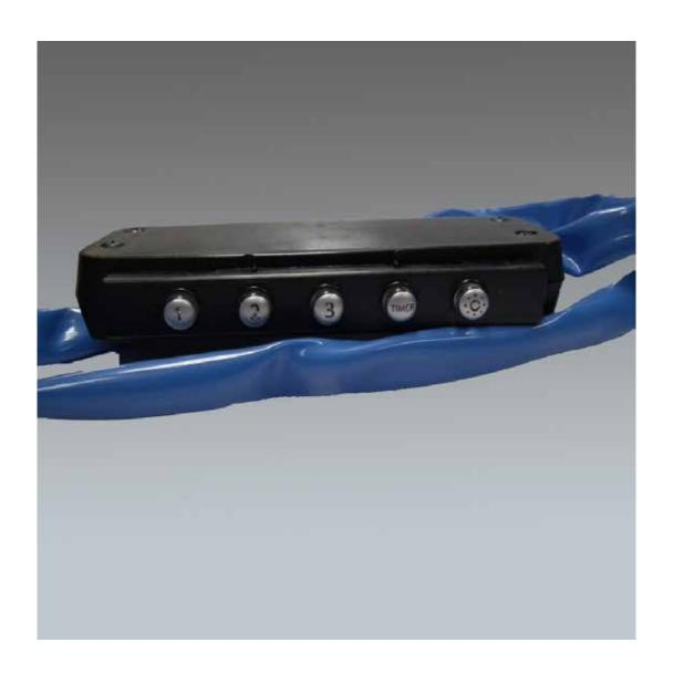
\*\*Please not if you are wiring a hard wired motor to a new switch unit you will need to check your old switch unit to find out which flex wires are attached to the appropriate speed settings. The different speed numbers can be found on the underside of the switch pcb. Do Not connect the same coloured wires together as this will blow the switch unit\*\*
