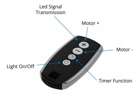
The cooker hood can be programmed to automatically switch off the turbine in up to 9 minutes. The timer is activated by pressing the button while the hood is running on the desired speed.
