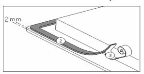
Stick the gasket (2) two millimeters from the external edge of the glass, after removing the protection tape (3).
