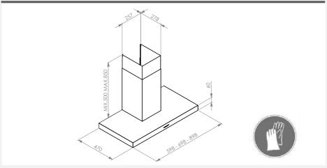
HOOD MUST BE INSTALLED ON MINIMUM 5" DUCTING OR RECTANGULAR EQUIVALENT
