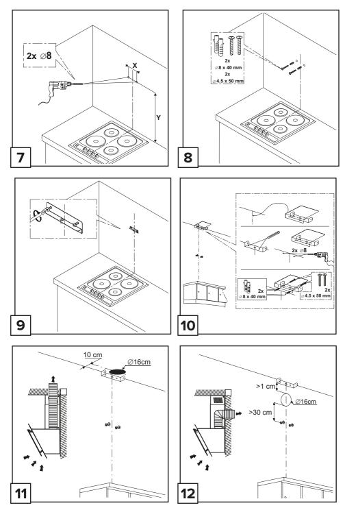
This hood must be installed on minimum 125mm round ducting or rectangular equivalent\*
