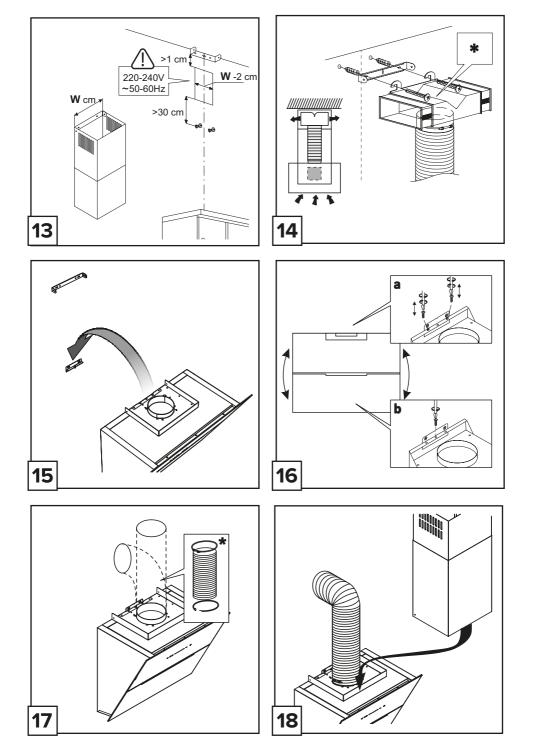
This hood must be installed on minimum 125mm round ducting or rectangular equivalent\*
