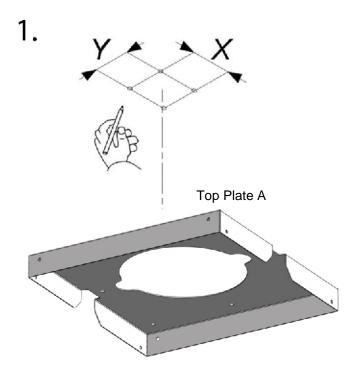
Use the top plate as a template to mark out you drill hole positions as above
