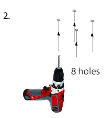
Drill and plug your holes. please note each installation is different so please ensure you have the correct fixings to the fixing material you are using.
