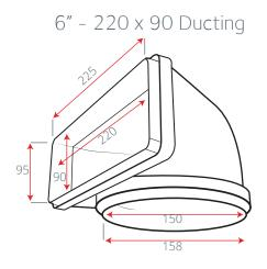
\*Please note adapters will not fit directly on to the motor exhaust.
