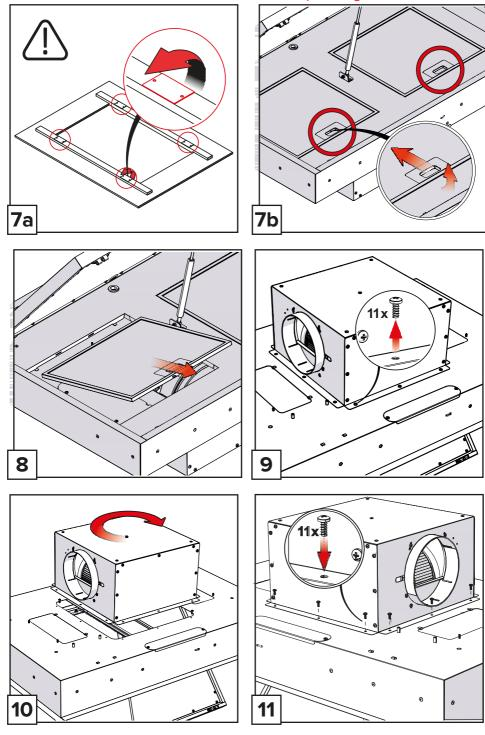
Hood must be installed on minimum 5" round ducting or rectangular equivalent Please remember to remove the motor flaps during installation
