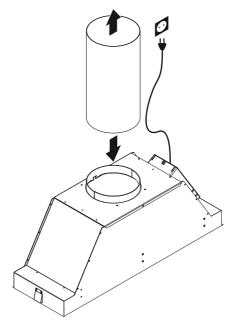
Please note this hood must be installed on minimum 6" / 150mm round ducting or rectangular equivalent
