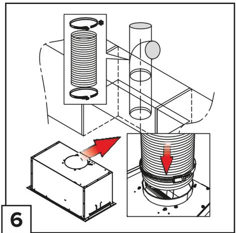
Must be installed on minimum 5" Round or rectangular equivalent ducting
