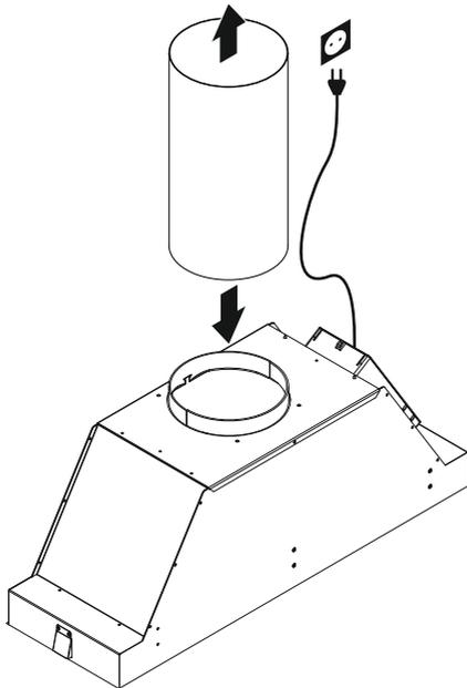
**Please note this hood must be installed on minimum 6" / 150mm round ducting or rectangular equivalent**
